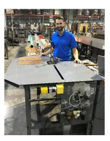
**Eutectic Welder:** Dustin modified the programming on one of the eutectic welders to increase efficiency by allowing the welders to be activated independently of each other. This project consisted of researching the capabilities of old controllers as well as wiring connections. The code also had to be re-written.
