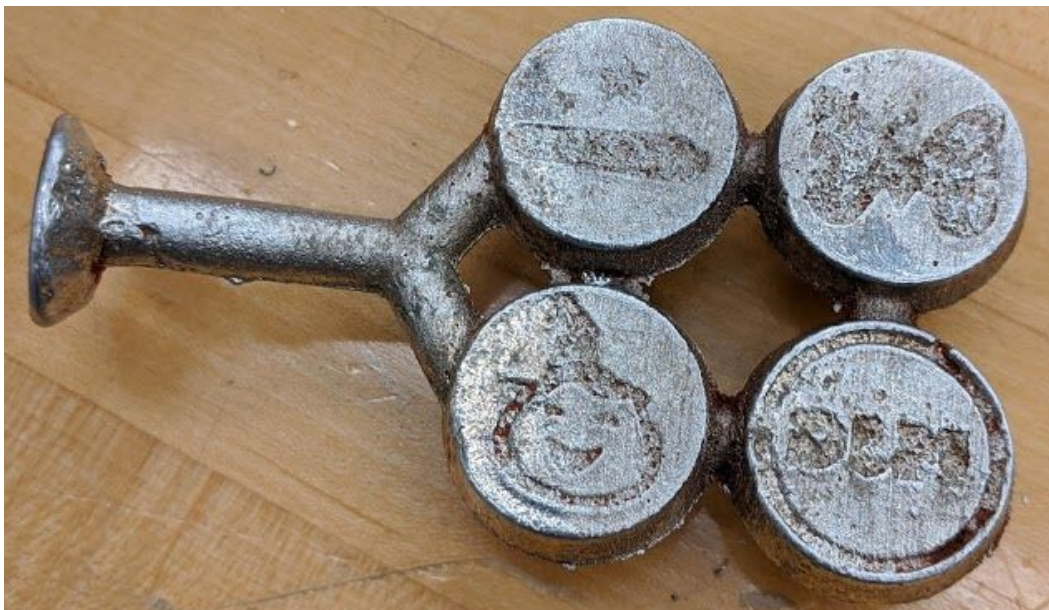
Figure 1. The figure above shows our sand casted seals before post processing
